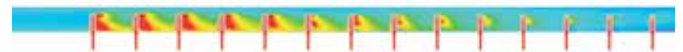
This CFD model shows a 4" dia. header with 14 nozzles. The total flow is 743 gpm (2813 lpm) at 2300 psi (159 bar). The model reveals the velocity leading into the first six nozzles exceeds the recommended maximum of 15 ft/s (4.5 m/s). In fact, the entry velocity for the first nozzle is 25.7 ft/s (7.8 m/s).
