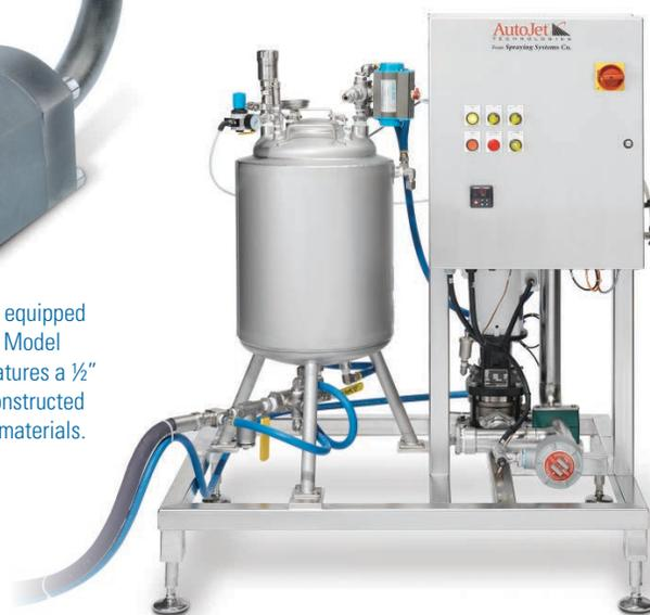
**AccuCoat Spray System** provides closed-loop temperature control for the sprayed liquid to enable the viscous liquid to be sprayed hydraulically rather than using compressed air for atomization. The spray controller also provides easy control of spray pressure and cycle times.
