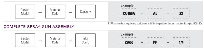
BSPT connections require the addition of a "B" in the prefix of the part number. Example: B22650.
