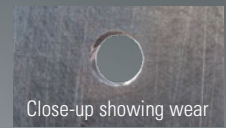
Worn SV Orifice Spraying Systems Co.: 10% increase in flow rate
