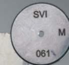
Worn SV Orifice Spraying Systems Co.: 10% increase in flow rate
