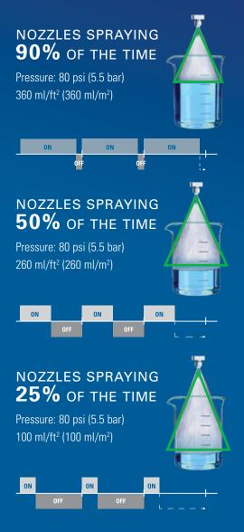
Note that the spray pattern remains unchanged when flow rate varies. This ensures consistent oil coverage on the strip.
