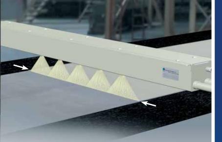
When zone 3 is activated, additional nozzles are turned off to accommodate ever narrower strip. In this example, two more nozzles have been turned off. Up to four zones can be configured.
