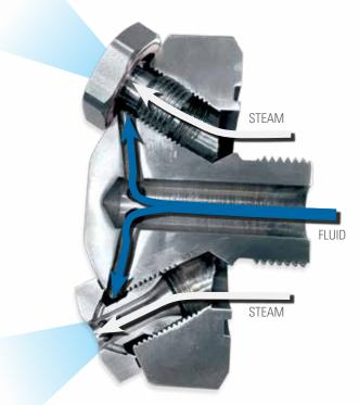
The mixing of steam and fluid just prior to exiting the nozzle orifices ensures tight drop size control.
