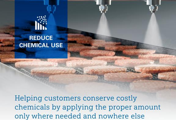
Many manufacturers are shocked to learn they may be able to reduce use of costly coatings by as much as 70% with precision application. Over-application and misting are the primary causes of coating waste. Our advanced spray technology delivers exceptional accuracy and consistency to ensure the proper amounts are applied and not one drop more.
